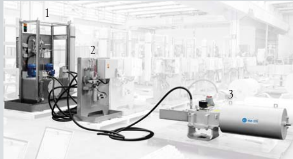
1. Hydraulic power unit 2. Control cabinet 3. RTQH actuator
